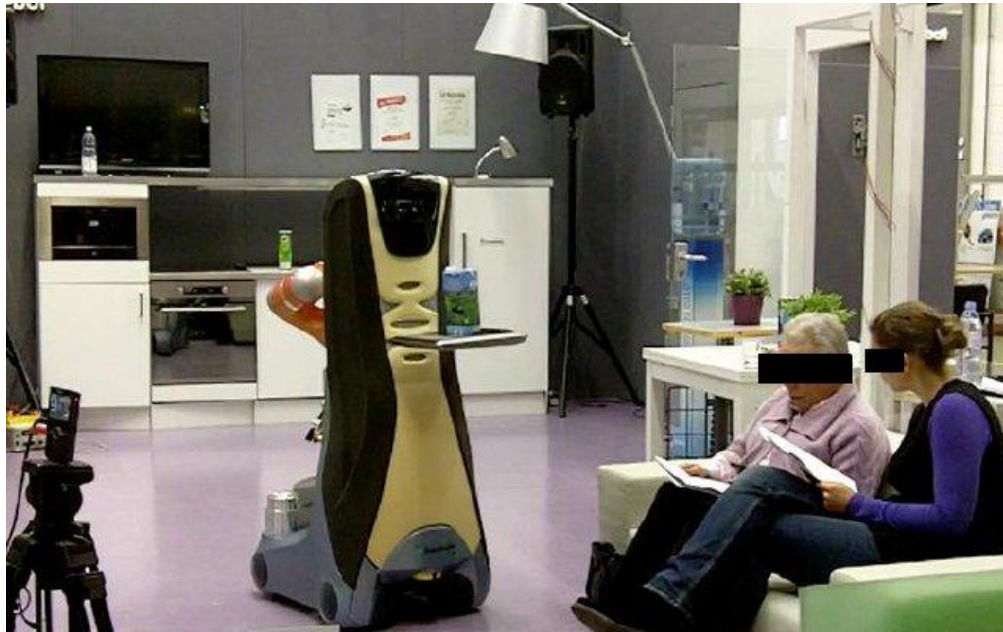
Figure 10: Robot got milk for the elderly based on the request sent from the smart phone (UI_LOC)
